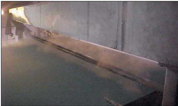
207" (5.25 m) fabric at 3600 fpm (1100 mpm) and 150 psi (11 bar) shower.
