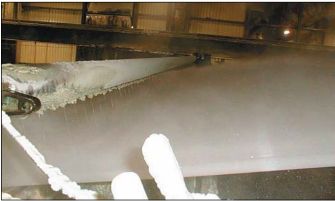
Fabric width of 251" (6.38 m) running 2800 fpm (850 mpm) with a shower pressure of 475 psi (33 bar).
