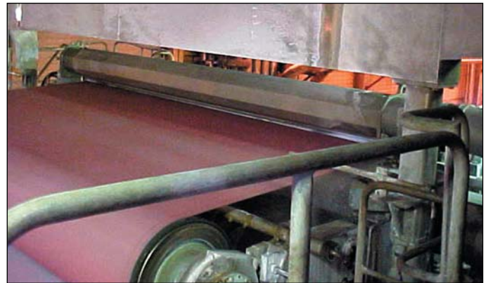
207" (5.25 m) fabric at 3600 fpm (1100 mpm) and 350 psi (25 bar) shower.
