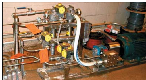
Unigy pumping system supplies shower water up to 5,000 psig (345 bar).
